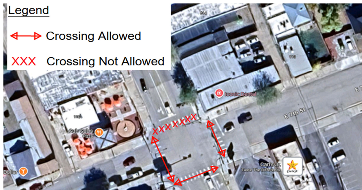
Figure 3-5. Removal of Pedestrian Crossing on North Leg of Intersection
